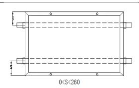
Installation of mounting beam through short side four pressure blocks
