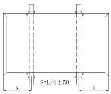
Installation of mounting beam through long side four pressure blocks
