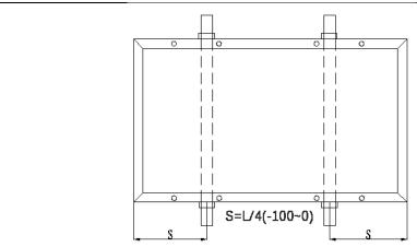
Installation of mounting beam through long side four pressure blocks
