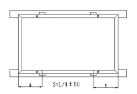
Installation of long side four pressing blocks embedded in beam
