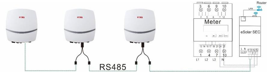
Figure 2: Ethernet cable splitter and cable connection
