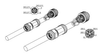
Figure 4.2 Thread the cables
