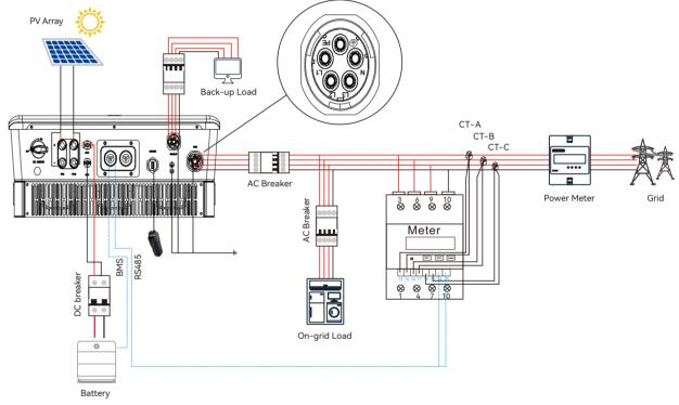
Figure 4.15 H2 Connection diagram
