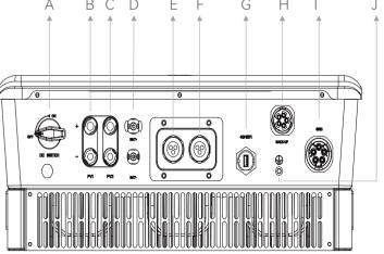
Figure 4.1 Electrical Interface of H2 inverter
