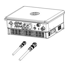
Figure 4.3 Connect the Cables
