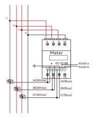
Notice: The hybrid inverter is with export limitation function, which can be realized by connecting SAJ recommended smart meter to the hybrid energy storage system. Users can contact SAJ for further details for the smart meters. If users have no intention to set the export limitation function, please ignore chapter 4.7.4.
