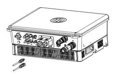
(2) Strip off the insulation skin of DC cable, the core is exposed to 10mm, and use a special tool to press the Battery Terminal.
