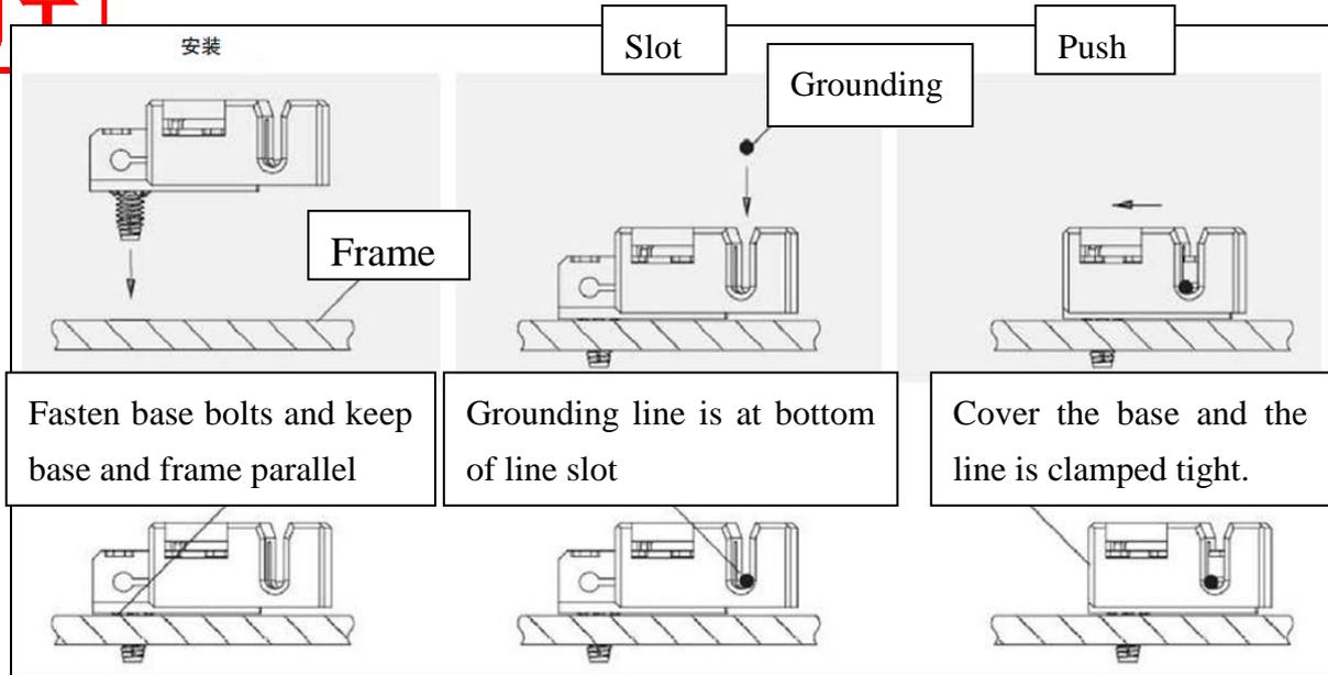
**Figure 11 Grounding Clamp Installation**
