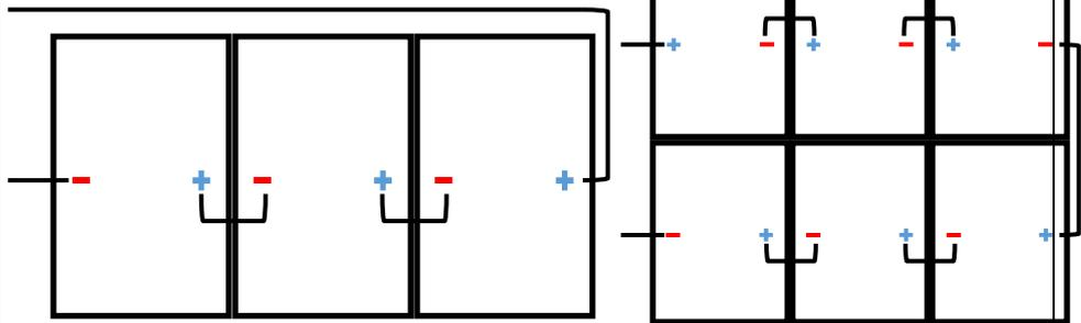
Note: An extension cord is required at the rotor head of the double row assembly and at the end of the single row.
