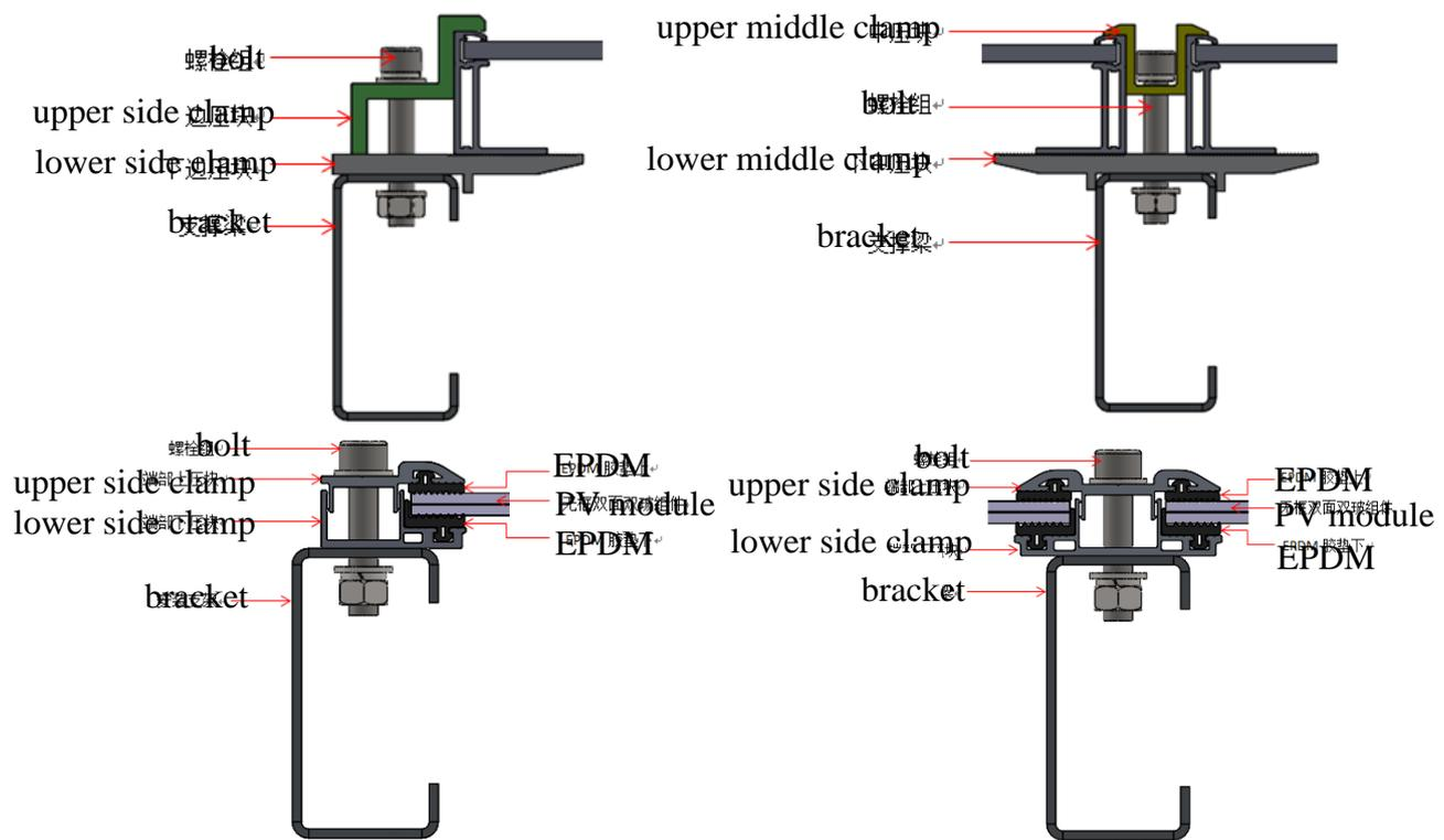
Figure 8 Clamp installation guideline
