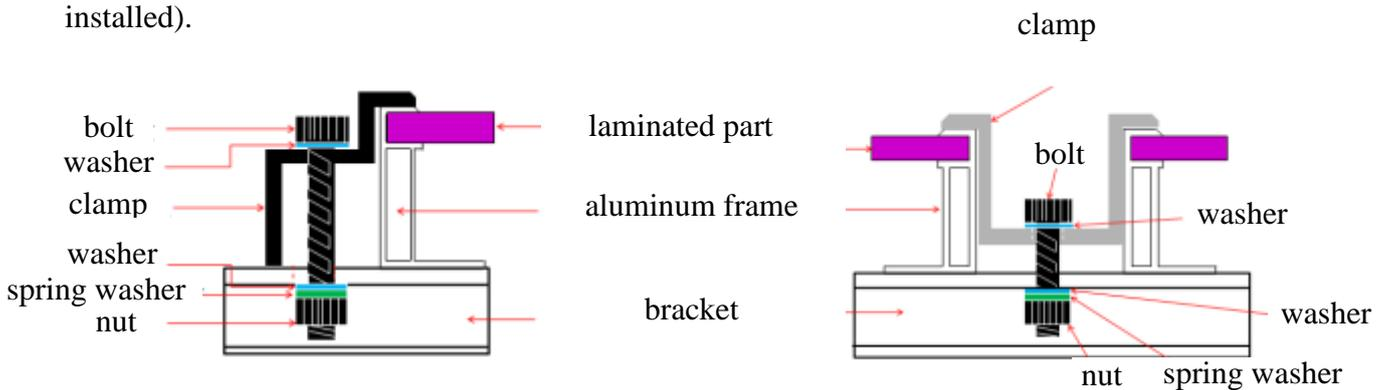
**Figure5 Clamp installation guideline**
