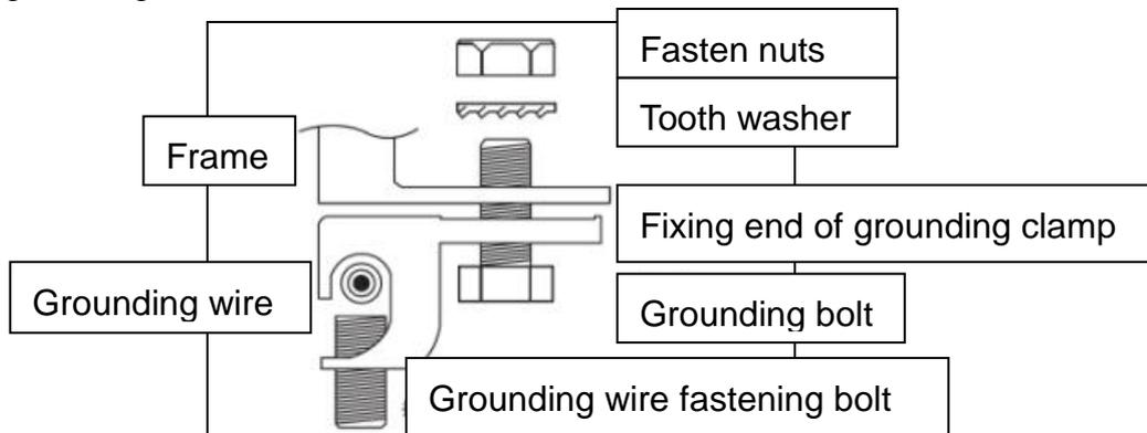
**Figure 12 Install Method**
