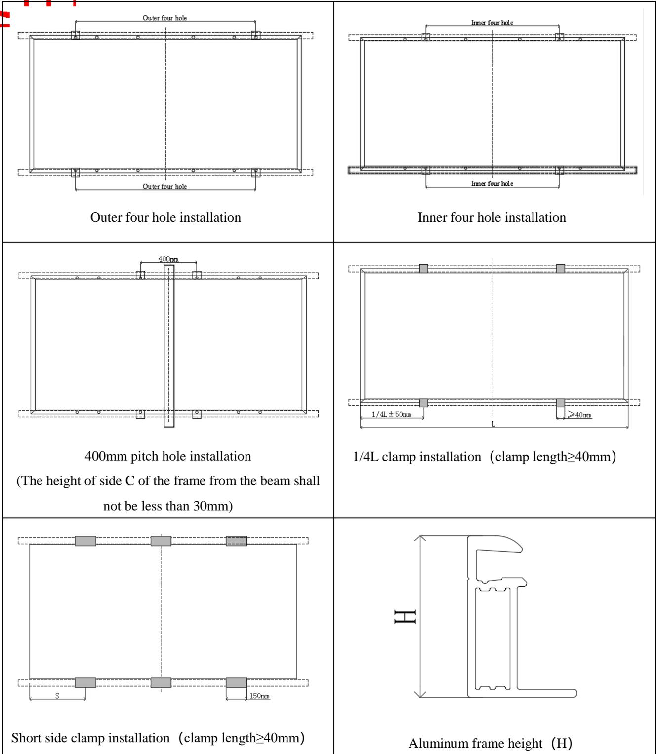
**Figure9 Bifacial component installation icon**
